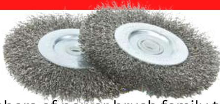
Wheel Brush is one of the members of power brush family that are mainly used for deburring. It is also used for surface finishing, edge blending, polishing, cleaning of paint, scale, rust and many more. Brush Firm manufactures wide range of wheel brushes ranging from large wide face wheel brushes to small diameter copper centre wheel brushes.
